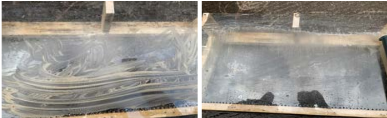
Figure 15.1: The Perspex “Solar Panel” Before Cleaning (Left) Figure 15.2: The Perspex “Solar Panel” After Cleaning (Right)
