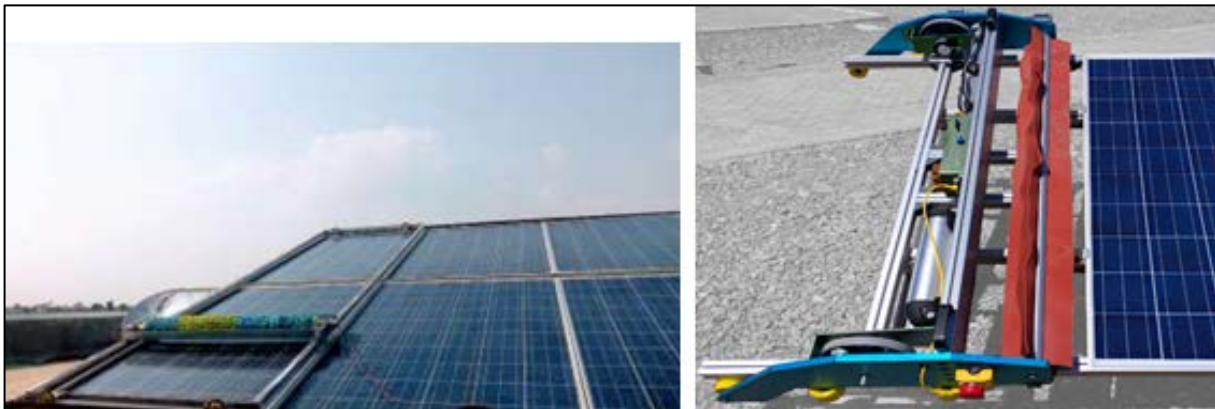
Figure 17.1: Mounted rolling brush solar panel cleaner (Parrott et al., 2018) (Left) Figure 17.2: Silicone rubber foam brushing device (Manju et al., 2018) (Right)
